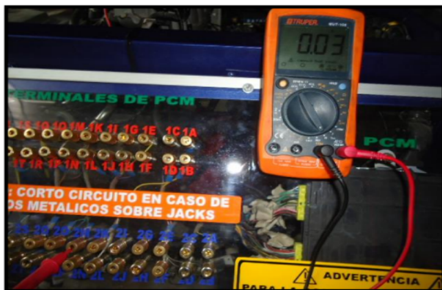
Figure 10. Voltage out of lower range TPS sensor
