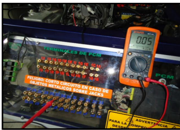
Figure 7. Voltage obtained by disconnecting the MAF sensor
