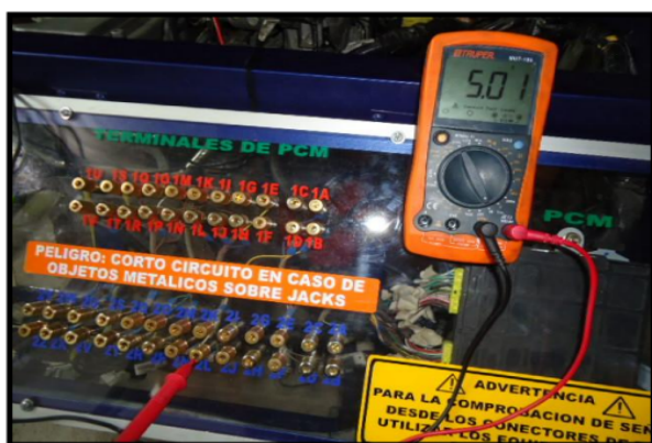
Figure 8. Voltage obtained by disconnecting the IAT sensor
